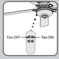
Note: The remote must be paired before the fan will operate.
